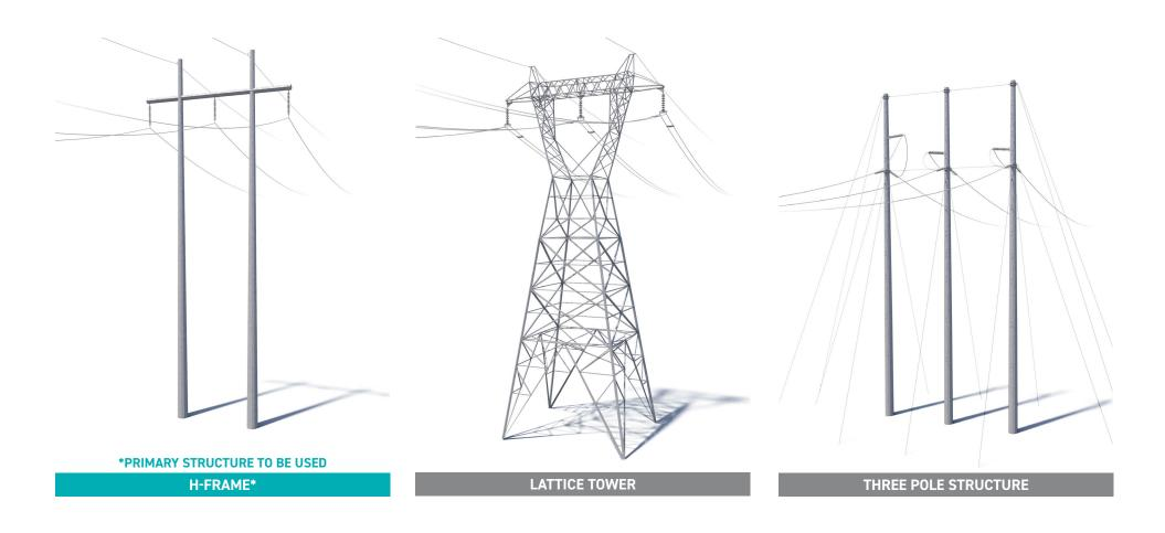
Crews plan to install steel H-frame, lattice tower and three-pole structures along the line route.
